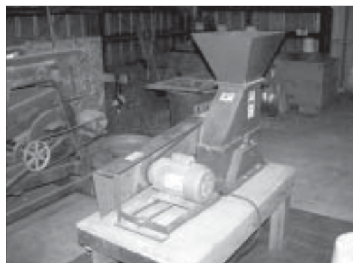
Speed King Hammermill model 615.
