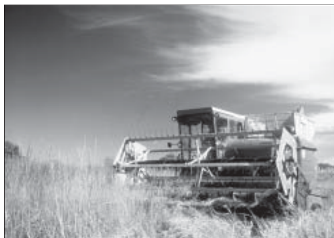
The Nature Conservancy's 1974 Massey Ferguson 510 combine with a grain head harvesting warm-season grasses.
