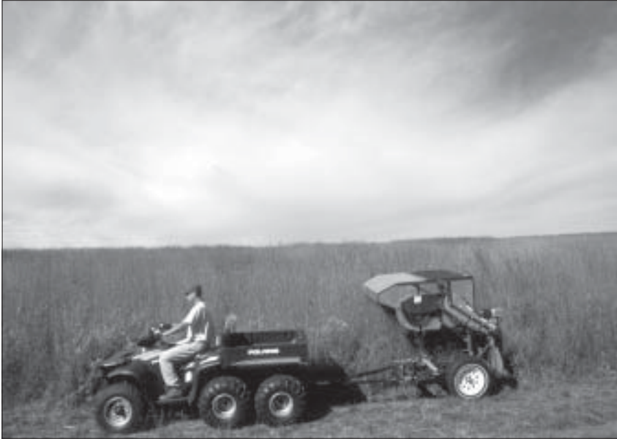
Collecting the seed of warm-season grasses using a seed stripper designed by Prairie Habitats, Inc.
