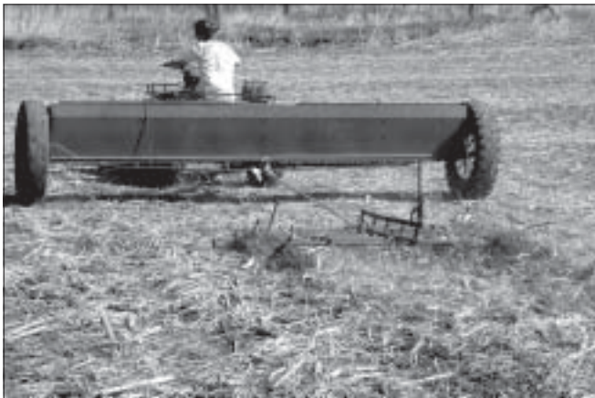
Pulling a harrow behind the E-ZEE Flow marks planter progress and incorporates some of the seed deeper into the soil.
