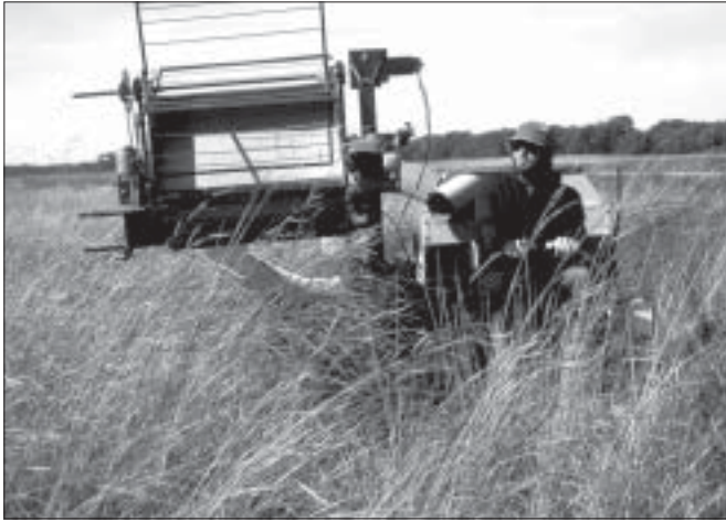
PPRI's custom fabricated seed harvester used during the early 1990s.
